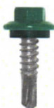
TEK Screws Self-drilling TEK screws for metal purlins. Lap TEK screws draw together joints and attach trim.
